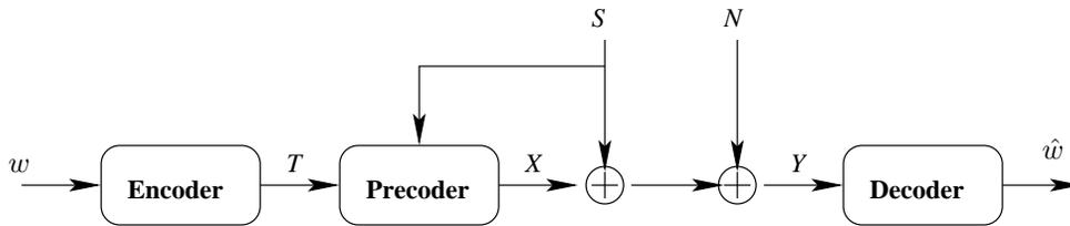
Fig. 8. General structure of a communication system for channels with causally-known discrete interference.
