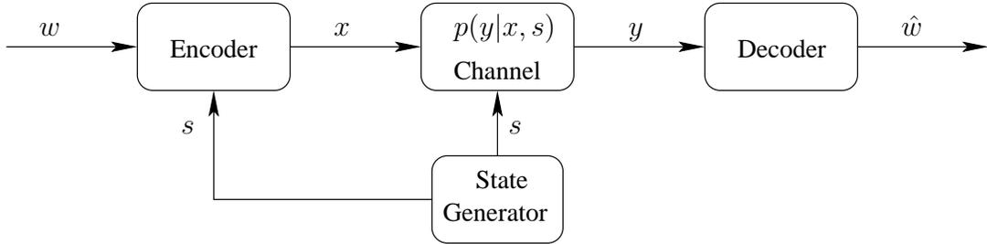
Fig. 1. SD-DMC with state information at the encoder.
