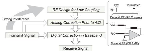
Fig. 2: Main components involved in self-interference cancellation.
