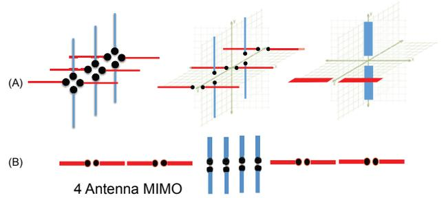
Fig. 7: Two and Three-dimensional antennas for MIMO structure.
