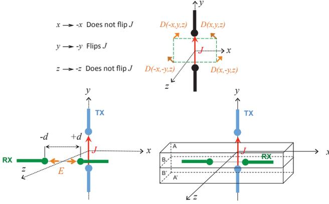
Fig. 5: Par-wise symmetrical antennas with input current ( $I$ ) in the  $y$ -axis direction. Net energy flowing out the whole region around the RX antenna is zero which results in  $S_{12} = S_{21} = 0$ .
