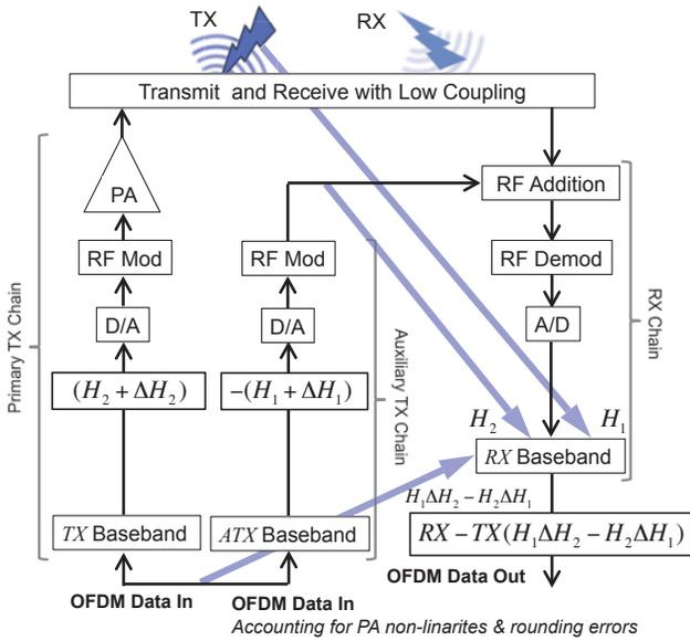
Fig. 3: Details of the self-interference cancellation.
