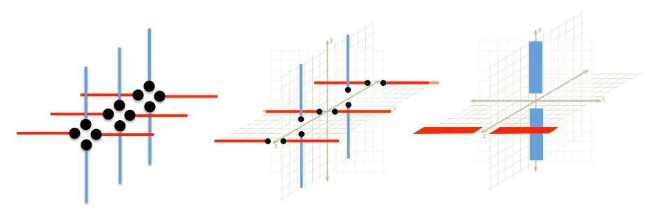
Antennas can be placed in any order, and can be of different lengths for multi-band operation.
